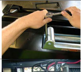
27. Fit the roller fair lead, pull only the end of the cable through and adjust the position of winch then bolt up to specified torque. For 9500 winch, use the 3/8"UNC x 1 ½" long bolts in the top and supplied 1 ¾" in the lower set through the RFL.
