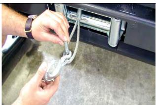
65. If winch fitted, fit off winch hook.
