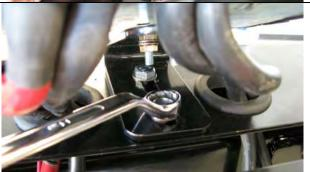
20. Using M8 fasteners fit control box mounting bracket to pan
