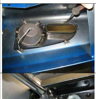
NOTE: Retaining bracket shown for clarity. Bolt holes at bottom
