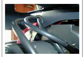
21. Insert grommets to winch bracket gusset holes and route cables through them as shown
