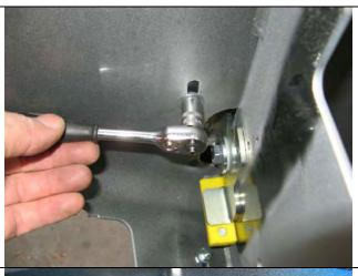
43. Slide the buffers down over the frame and secure using M6 flange nuts on the four lower buffer studs on each buffer and M6 nyloc nuts with large M6 flat washers on the two studs located on top face.
