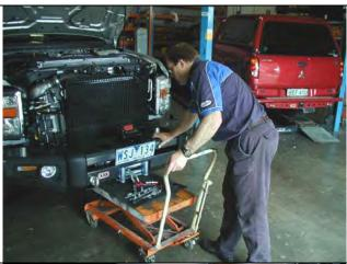
59. Using two people, three if winch fitted, position the bar assembly on the vehicle mounts.
