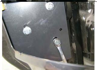
61. When bar is aligned, tighten bolts to specified torque.
