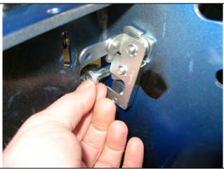
46. Fit the striker pin to the *RHS* hinge plate and secure with 5/16"UNC nut and spring washer as shown and tighten to 22Nm or 16lbft
