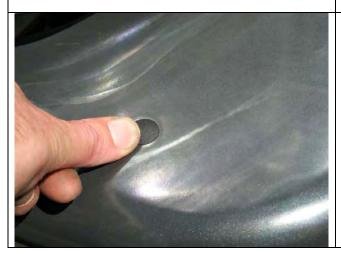
69. Unless fitting CB aerials, fit blanking plugs in provided holes in the top of the wings.
