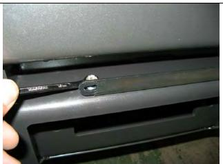
17. Secure the number plate bracket using M6 bolts, flat washers and flange nuts. Attach the longer side to the bullbar and the shorter side to the number plate.
