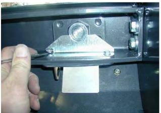
16. When the large nut is in its final position, fit the retaining bracket and optional bottle opener as shown and secure using M6 bolt, washer and flange nut sets.
