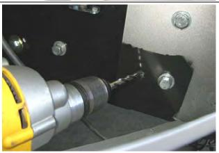
62. Using the M10 pilot holes in mount brackets, drill pinning hole through uprights on bull bar. Fit M10 screw, washer set and flange nut and do up tight.
