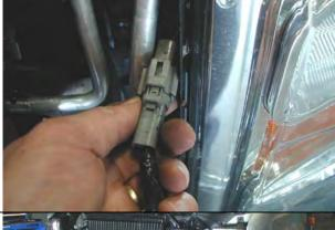
If fog lights fitted in bumper, undo fog light loom connection (connection located on LHS of vehicle behind headlamp)
