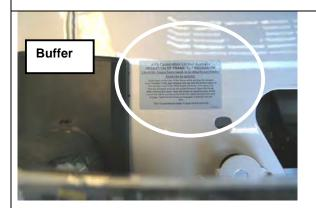
66. Apply the frame tilt operation label to the top face of the pan adjacent to the buffer as shown in diagram
