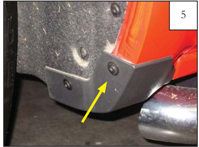
Using a T-15 Torx bit, remove two factory screws in mudguard at rear of front wheel well and remove mudguard.
