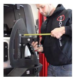
9. Lengthen the tailgate link, then close the gate and install the 1/2" x2 bolt. You may need to use a punch to line everything up. Tighten the link until the rubber isolators touch the tailgate plate. Note that the rubber isolators may need to be shimmed out using washers. This all depends on how the bumper is positioned. Once adjusted, open the gate and tighten the jam nuts on the link.
