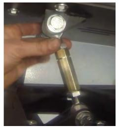
10. - OPTIONAL- If installing the optional hi-lift mount, place the mount onto the carrier and loosely install the (4) 5/16" button head bolts. Using a 3/16" allen, tighten up the (4) bolts. Next, install the 7/16" bolts that will hold the hi-lift. Using a socket and hammer, tap on the retaining clips. Now that your bolts are in place, insert the jaw of the jack into the carrier and install the wing nuts, then tighten them down
