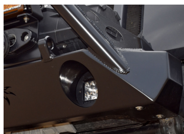
Recessed light buckets accept OEM fog lamps or LED cube lights (with adapters)
