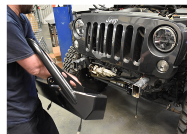
Installation requires frame modifications to achieve best approach angle
