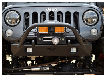
BFH™ II is slightly wider than the Jeep’s frame, for maximum clearance
