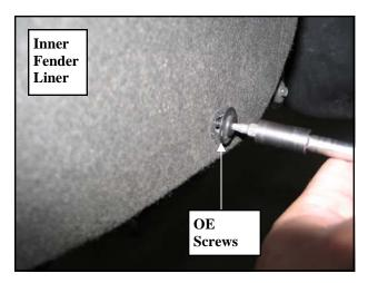
3. Remove the (3) bolts and remove the **OE** inner fender bracket from the vehicle. Save the **OE** bolts for reinstallation.
