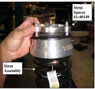
22. Install the strut assembly into the strut tower and secure using the supplied **10mm** flange nuts. Leave the bolts hand tight only at this point.
