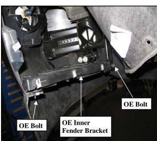
4. Remove the (7) **OE** nut-clips from the from the **OE** inner fender bracket and install them onto the new inner fender bracket (94-10299 drvr and 94-10300 pass).
