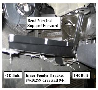
6. Mark the front bumper and valance for trimming using masking tape. Follow the contour of the inner fender starting approximately **16**" up from the bottom of the valance, **7**/**8**" in from the bottom of the bumper, and **1.5**" in from the edge of the lower valance.
