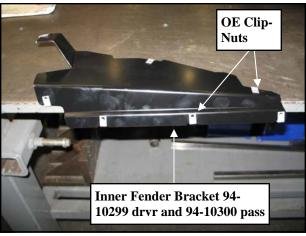
Install the new inner fender bracket (94-10299 drvr and 94-10300 pass) to the OE mounting location and secure using the previously removed (3) OE bolts.
