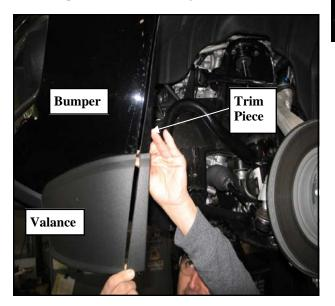
8. Trim the lower rear section of the inner fender liner to provide tire clearance. Use the dotted line as a guide line for trimming.
