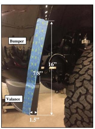
7. Using a suitable cutting tool, trim the front bumper and valance along the cut line.
